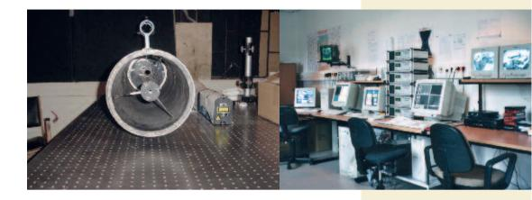
This group, led by Edgar Alfonso, works very closely with the Classical Foundations of Physics Group in a project to detect potential variations of light velocity during the year. The project uses a high definition Michelson interferometer for systematic measurements.
